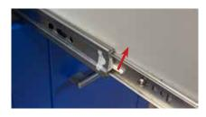
With drawer fully extended, locate slide release tab on left side and push up to release.
