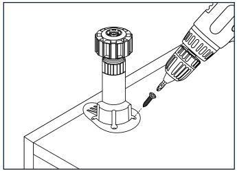
2. Place the 2 back leg brackets 1" from the back edge with the support plate overlapping the end panel – 1/4" from the outer edge.
